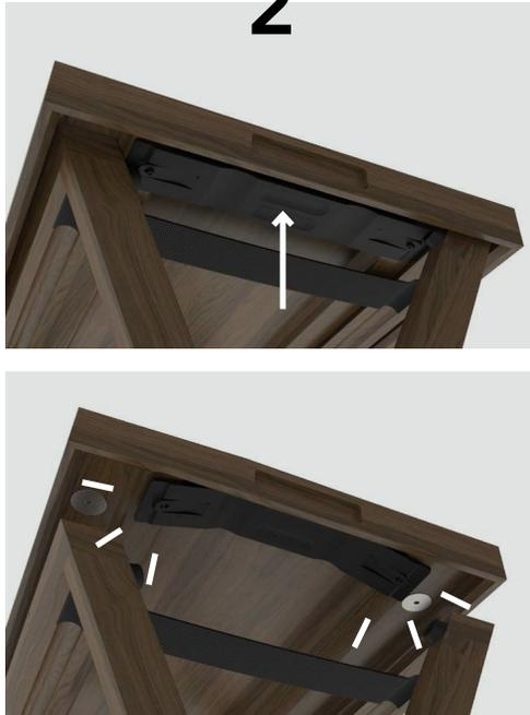
Depress the tab underside to separate magnets and demount
